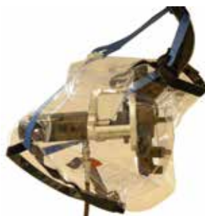
Example of a hydraulic tool fitted with safety guard and safety strap.
