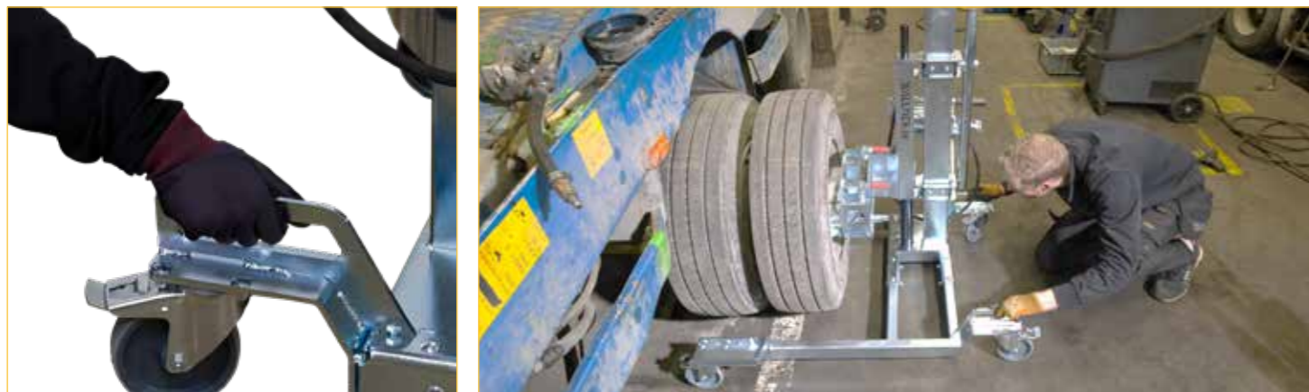
The rear handles provide extra support when installing the hub onto the wheel axle
