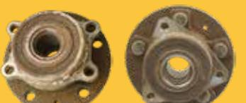
1. Dismantling 3-4 bolted wheel bearing/hub.
