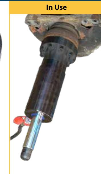
This tool allows removing the hub from the axle, even if it is heavily rusted and seized. This method simplifies and severely minimizes the labor time when replacing the front wheel bearings. No need to cut the hub or crack the knuckle in the shop press anymore. Fits models from 2005 - ... with 9 holes in the brake disc/rotor. 9 pcs hex bolts for safe removal are included in the set.
