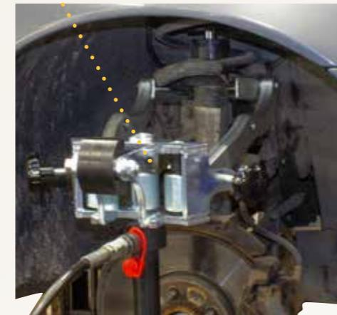
3. The upper frame can be mounted upside-down and be used as a lifting jack when working with other jobs on the suspension system.
