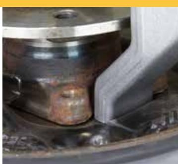
The press feet get access to the small surfaces close to the bearing, pressing on the knuckle behind the brake shield.
